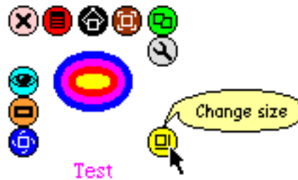
Figure 5: TestMorph with its halo. The cursor has lingered over a handle for a few seconds, causing the help balloon to appear. Moving the cursor away from the handle will cause the balloon to disappear. Clicking on the background will make the halo itself go away.
