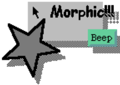
Figure 7: A composite morph created by embedding various morphs in a rectangle morph. The composite morph is being moved. The embedded morphs stick out past the edge of the rectangle, which is reflected by the drop shadow.
