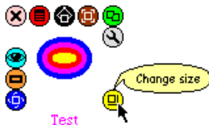
Figure 5: TestMorph with its halo. The cursor has lingered over a handle for a few seconds, causing the help balloon to appear. Moving the cursor away from
