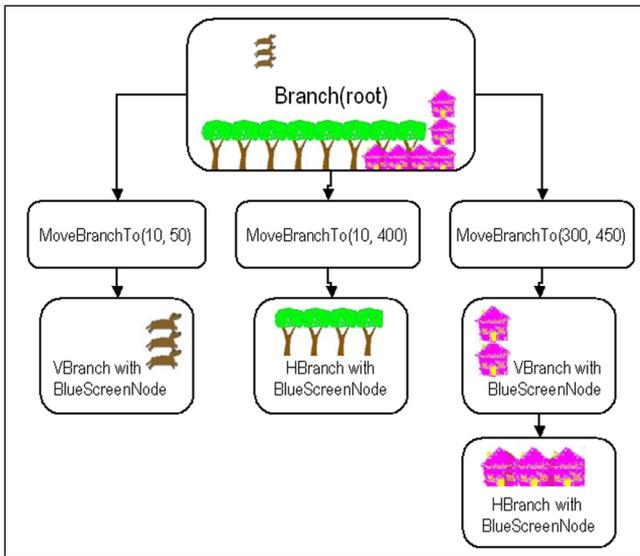
Figure 1: An example of class material: a scene graph of an animation, decomposing a scene into a tree of elements.
